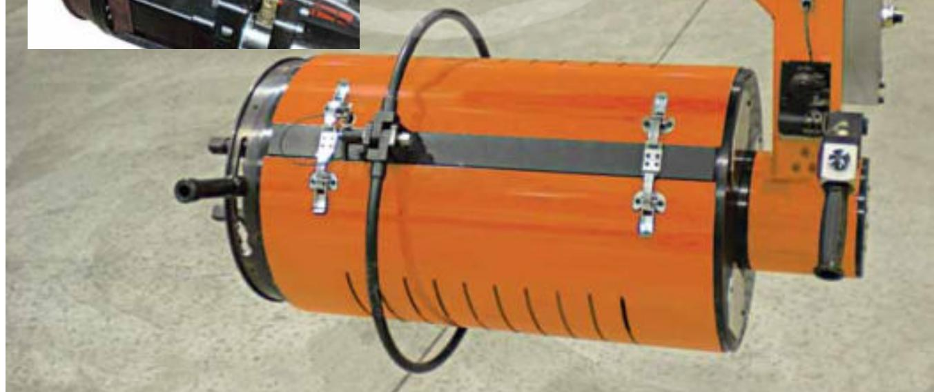
***The above manually operated railroad wheel bearing multiple has the capability to tighten three (3) fasteners equally spaced on various centers between 3.50" to 5.85" diameters up to 600 NM torque.***
