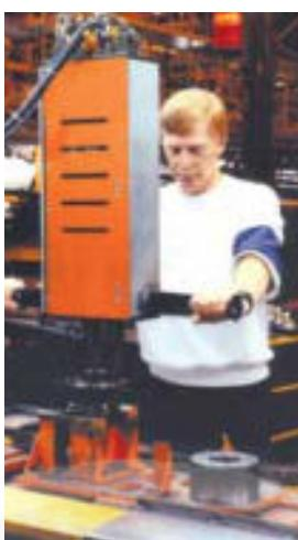
*Repair bay operator is using a two spindle fixture tool to fasten components of a wheel hub assembly.*
